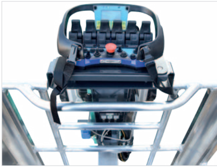
User-friendly control panel with external support to the basket. More space available in the basket.
